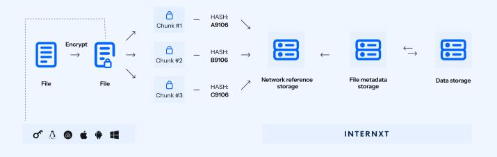
User's device Windows, macOS, Linux, Android or iOS Internxt internal API Product API (Drive, Photos, Send) Network API OVHcloud network & storage Erasure coding technique ensures files integrity when sent to OVH for storage
